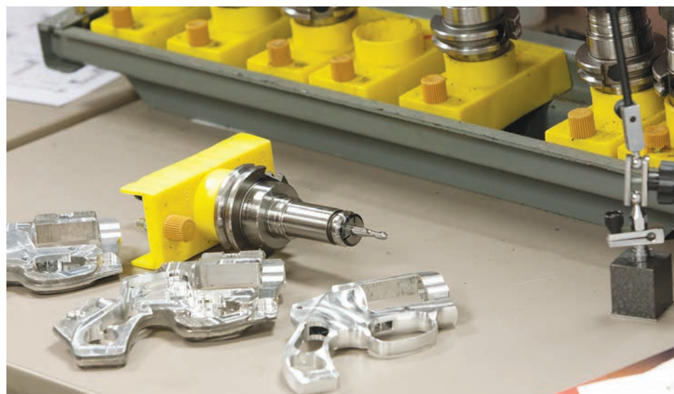
Smith & Wesson uses end mills secured in REGO-FIX powRgrip toolholders for the various stages of machining aluminum pistol frames.
