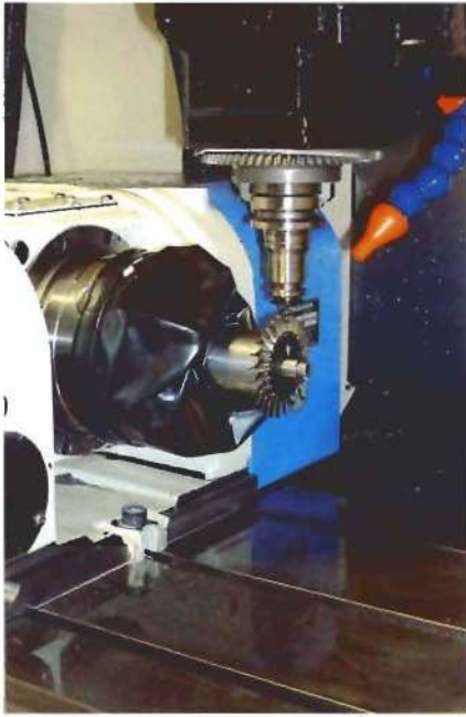
Turbine wheel production: The company uses super alloys with relatively high nickel and cobalt content, which are extremely difficult to machine. Pictures: Jakadofsky / Rego-Fix
