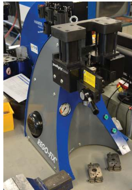
APN placed its powRgrip tool-changing unit near its high speed machines that use the toolholders.
