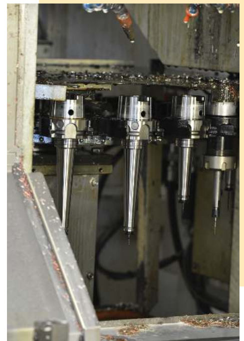
The powRgrip toolholders virtually eliminate vibrations, allowing for tighter high concentricity with deviations of less than three microns.
