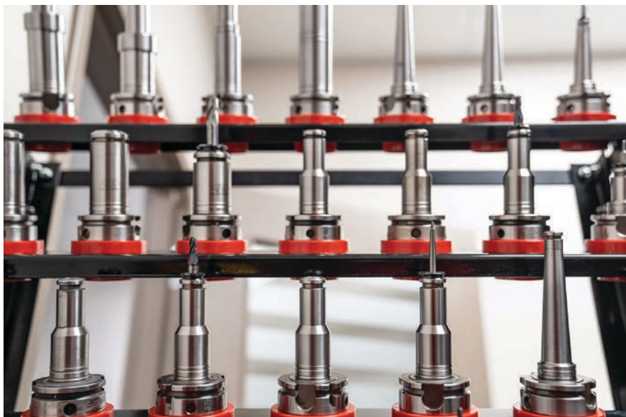
Rego-Fix powRgrip toolholders provide gripping force with TIR of less than 0.0001” ( \leq 3 \mu\text{m} ) and length adjustment repeatability of less than 0.0004” (10 \mu\text{m} ).
