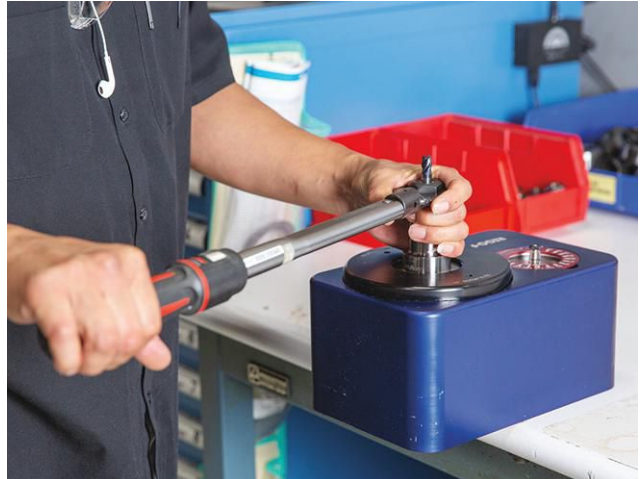
The Torco-Block benchtop tool assembly assistant unit features a built-in torque meter and interchangeable indicator rings for different ER series holders, saving the shop's torque wrenches from damage.
