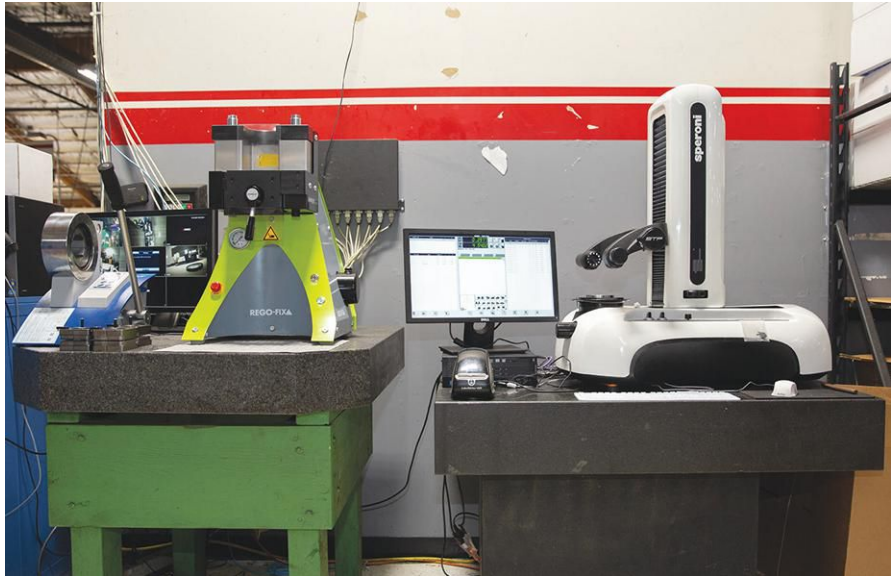
Rego-Fix powRgrip toolholding units take less than 10 seconds to press in a tool or remove it from the toolholder. Because no heat is used in the process, tools can be used immediately after a tool change.
