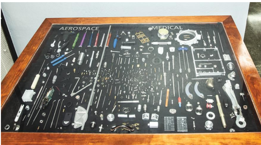
Medical and aerospace parts produced by Precision Swiss Products with tolerances as tight as \pm 0.00015 " (0.0038 mm) have intricate, complex geometries that can require as many as half a dozen operations with very small tools.
